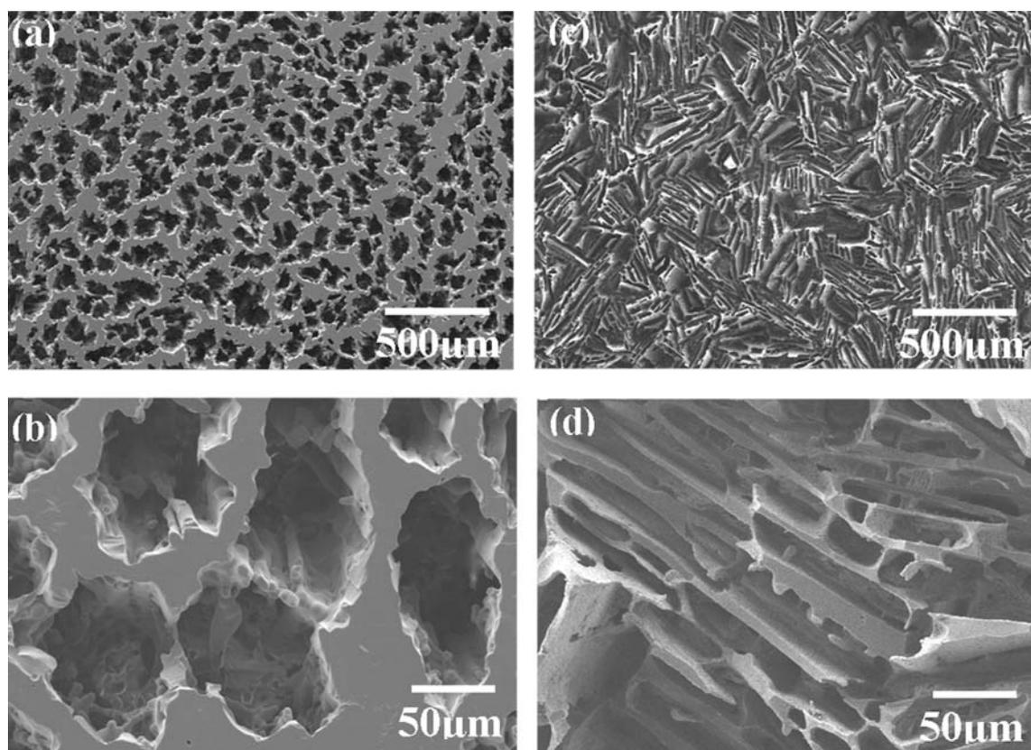
**Figure 1.** SEM images of the cross sections of 13-93 bioactive glass scaffolds prepared with different microstructures from suspensions containing 15 vol % particles: (a,b) columnar microstructure (solvent: water + 60 wt % dioxane); (c,d) lamellar microstructure (aqueous solvent). The cross sections are perpendicular to the freezing direction.
