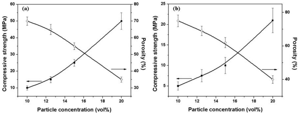
**Figure 2.** Compressive strength (in the direction of pore orientation) and porosity of 13–93 bioactive glass scaffolds with (a) columnar microstructure and (b) lamellar microstructure, prepared from suspensions containing different concentrations of particles.
