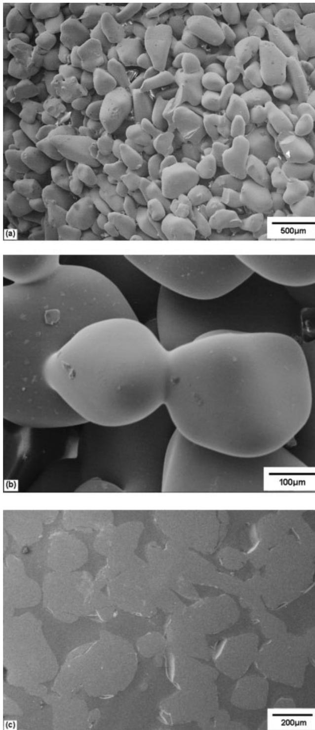
**Figure 2.** SEM of (a) the surface of a porous glass construct prepared by sintering, (b) the neck region between two particles, showing bonding between the particles, and (c) a cross-section of the construct showing the bonded particles and pores.
