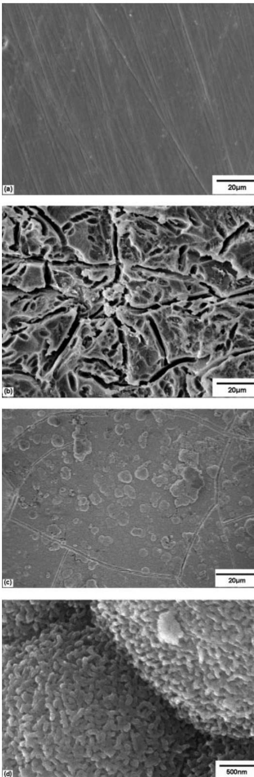
**Figure 8.** SEM of (a) the surface of 13-93 glass, and the surface after immersing the glass in a simulated body fluid for 1 day (b), and 7 days (c). A high magnification micrograph of the surface (7 days immersion) is shown in (d).
