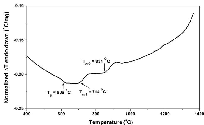
**Figure 1.** Differential thermal analysis of 13–93 glass, showing the glass transition and crystallization regions.
