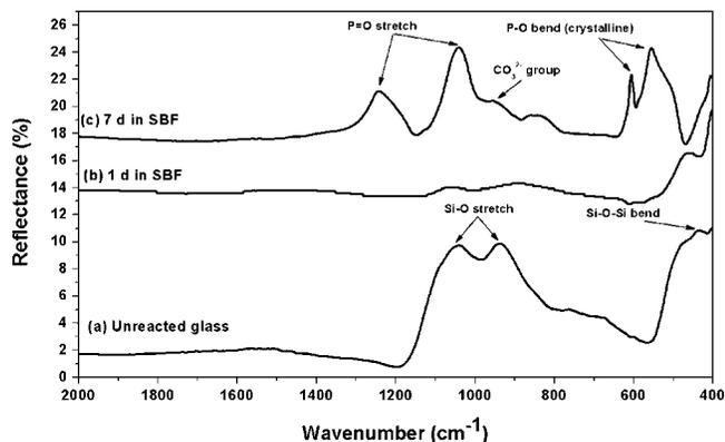
**Figure 5.** FTIR of the 13-93 glass and the glass after immersion in a simulated body fluid at 37°C for various times.
