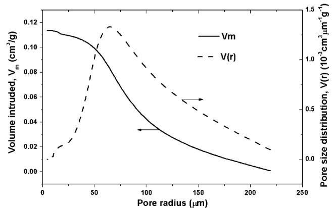
**Figure 3.** Mercury porosimetry of the fabricated constructs, showing the pore volume and the pore size distribution as functions of the pore radius.
