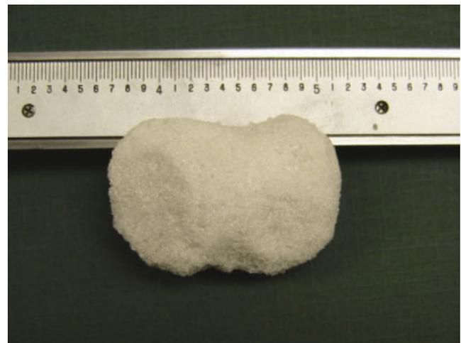
**Figure 9.** Optical micrograph of a porous construct with the shape of the articulating surface of a human proximal tibia prepared by slip casting and sintering 13-93 glass particles. [Color figure can be viewed in the online issue, which is available at [www.interscience.wiley.com](http://www.interscience.wiley.com).]
