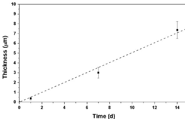
**Figure 7.** Thickness of the hydroxyapatite layer formed on the 13-93 glass as a function of the immersion time in a simulated body fluid at 37°C. (Linear regression:  $r = 0.9954$ ;  $p < 0.0001$ ).
