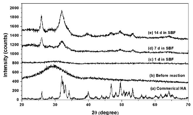
**Figure 4.** Thin-film XRD of the 13-93 glass, and the glass after immersion in a simulated body fluid at  $37^\circ\text{C}$  for various times.
