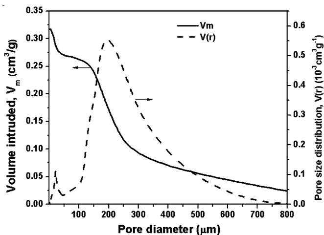
Fig. 5. Mercury porosimetry data for the pore volume and pore size distribution vs. pore radius, for the fabricated 13-93 glass scaffolds.
