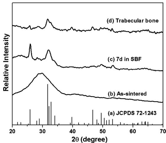
Fig. 8. X-ray diffraction patterns of: (a) reference hydroxyapatite (JCPDS 72-1243); (b) porous 13–93 glass scaffold in the as-sintered condition; (c) sintered 13–93 glass scaffold after immersion in a simulated body fluid for 7 days; and (d) human trabecular bone.
