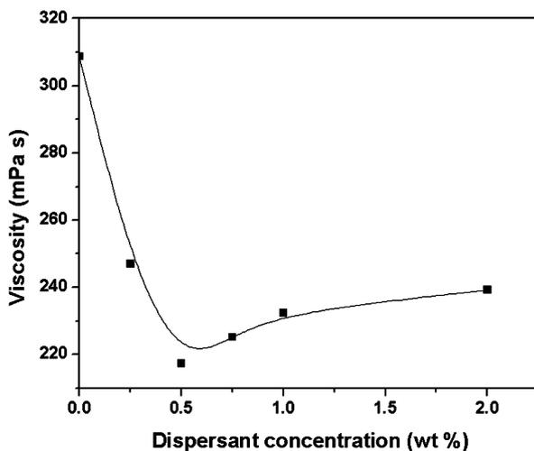
Fig. 2. Viscosity of aqueous suspensions containing 35 vol.% 13–93 glass particles vs. dispersant concentration (shear rate =  $100 \text{ s}^{-1}$ ).
