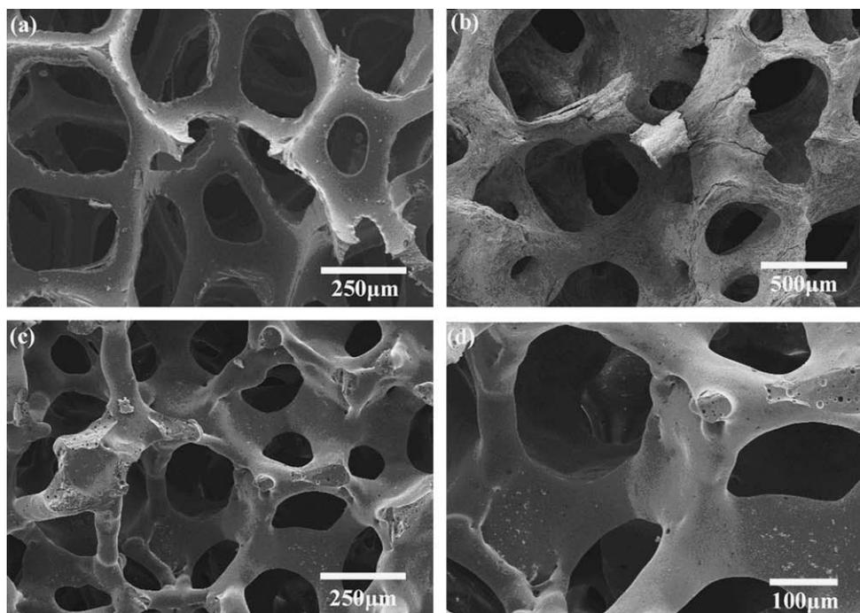
Fig. 4. Microstructures of: (a) polyurethane foam used in the experiments; (b) dry human trabecular bone; and (c, d) 13-93 glass scaffolds fabricated by a polymer foam replication technique.
