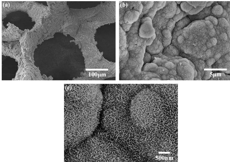
Fig. 7. SEM images of the surface of a 13–93 glass scaffold after immersion for 7 days in SBF: (a) lower magnification image; and (b, c) higher magnification image showing fine needle-like hydroxyapatite crystals.
