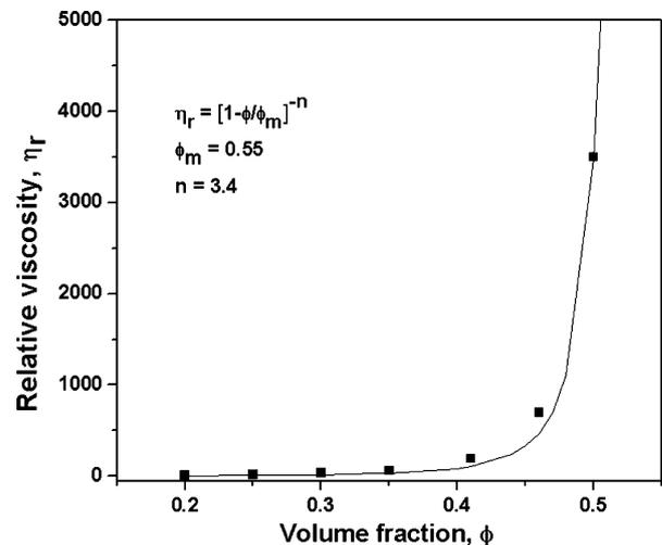
Fig. 3. Relative viscosity vs. volume fraction of 13–93 glass particles in aqueous suspensions stabilized with 0.5 wt.% EasySpense (shear rate =  $100 \text{ s}^{-1}$ ).
