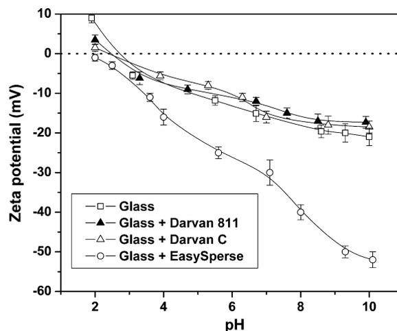
Fig. 1. Zeta-potential of 13–93 glass particles vs. pH, for suspensions without dispersant and for suspensions containing 1 wt.% Darvan 811, Darvan C or EasySperser.
