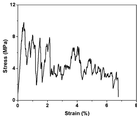
Fig. 6. Stress-strain response of porous 13-93 glass scaffolds in compression.
