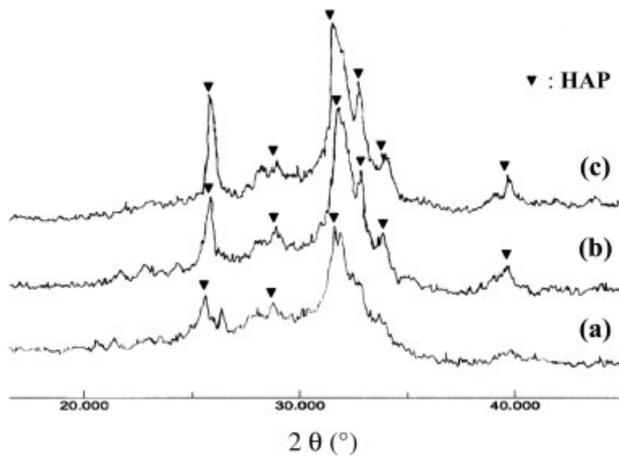
**Figure 2.** XRD spectra of GBC after different immersion time.
