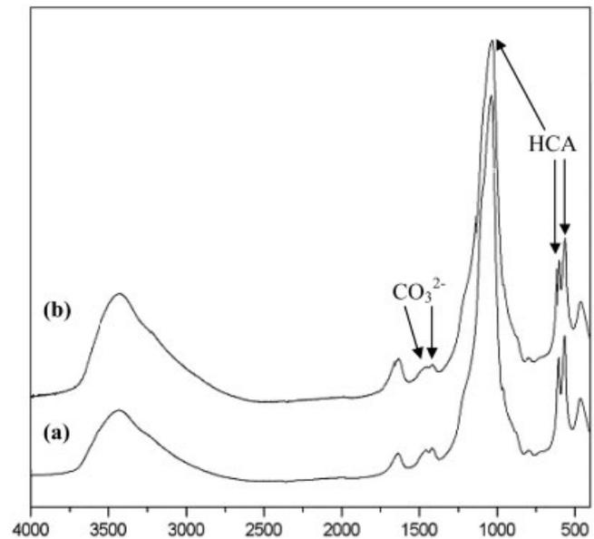
**Figure 4.** FTIR spectra of bone cement after 7 days immersion time.
