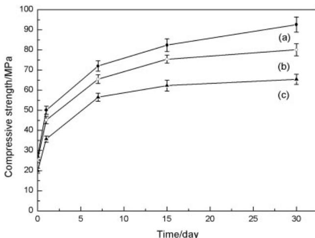
Figure 5. Compressive strength of bone cement after different immersion time. (a) GBC; (b) GBNHAPC; (c) GBMC.
