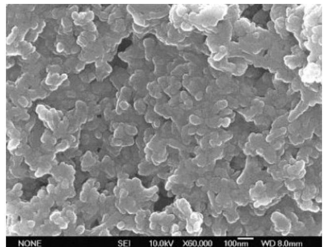
Figure 6. SEM pictures of as-dried nanoscale HAP crystallite.
