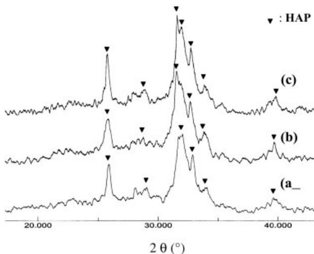
**Figure 3.** XRD spectra of GBNHAPC after different immersion time.
