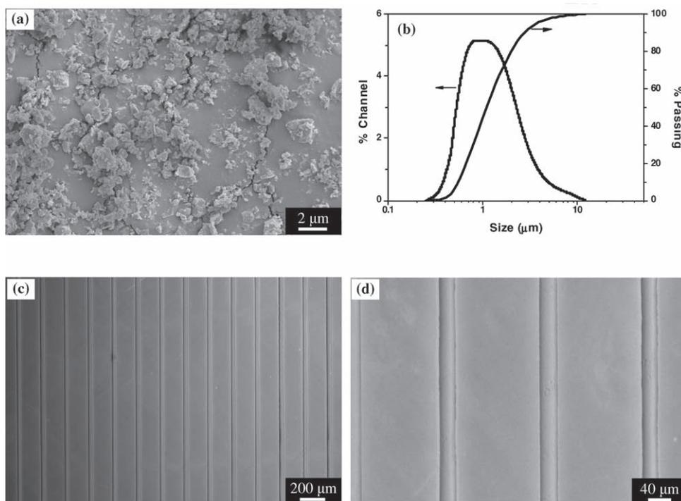
**Figure 1.** 6P53B glass particles used in the present work: a) SEM images of glass particles after attrition milling; b) the particle size distribution; patterns printed through 30  $\mu\text{m}$  capillary tip using the hydrogel-based glass ink; c) as-printed parallel filaments; and d) high-magnification image of the filaments.
