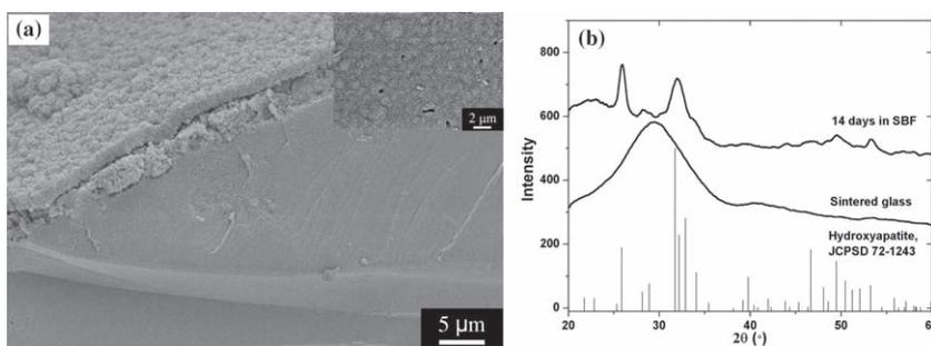
**Figure 4.** Surface reaction layer of 6P53B glass scaffold after immersion in simulated body fluid (SBF) for two weeks. (a) SEM images showing the glass filament covered with fine nanosized hydroxyapatite crystals (inset showing detailed morphology of the crystals); (b) X-ray diffraction pattern of the formed crystals.
